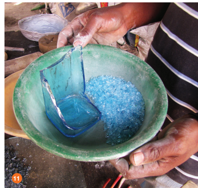
Fig 8 Making bead moulds... Fig 9 ...lots of bead moulds! Fig 10 Crushing bottles.... Fig 11 ...into powder glass! Fig 12 Filling a star bead mould with a mixture of blues. Fig 13 Loading the kiln with moulds using a very long handled spatula as protection from the heat Fig 14 The transformation of old glass into new beads! Moulds in the kiln resting on old car springs
