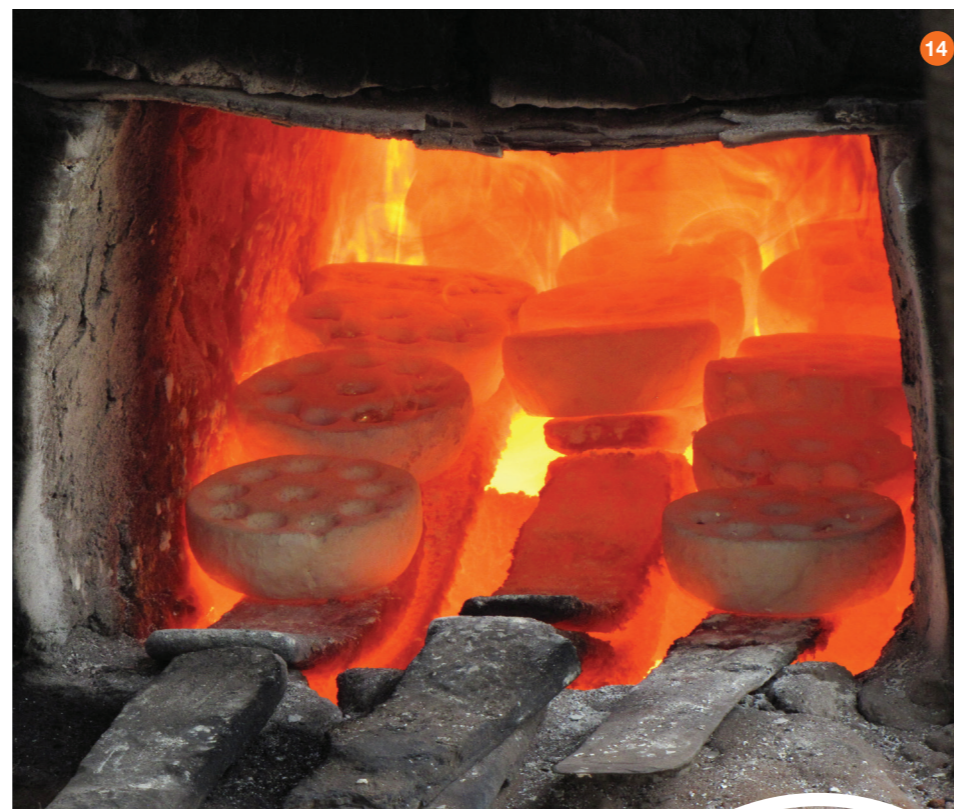
Fig 8 Making bead moulds... Fig 9 ...lots of bead moulds! Fig 10 Crushing bottles.... Fig 11 ...into powder glass! Fig 12 Filling a star bead mould with a mixture of blues. Fig 13 Loading the kiln with moulds using a very long handled spatula as protection from the heat Fig 14 The transformation of old glass into new beads! Moulds in the kiln resting on old car springs
